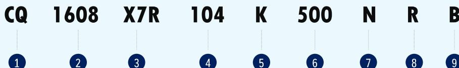
① Monolithic Multilayer Ceramic Capacitor Leadless Type for Automotive Application
